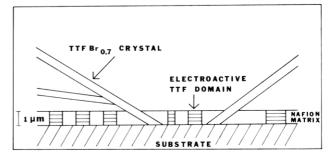
Figure 11. Diagram of the cross section of a Pt/NAF,TTF<sup>+</sup> electrode.
