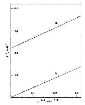
**Figure 7.** Plot of the reciprocal limiting current vs. the reciprocal square root of  $\omega$  for the reduction of Fe(CN)<sub>6</sub><sup>3-</sup> on (a) Pt/NAF,TTF<sup>+</sup> electrode, (b) bare Pt electrode. The solution is 10 mM Fe(CN)<sub>6</sub><sup>3-</sup>, 1 M KBr. Currents are recorded at 0.0 V. Electrode area is 0.458 cm<sup>2</sup>.
