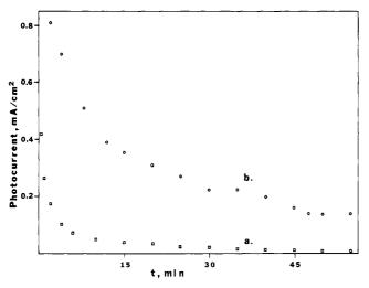
Figure 13. Photocurrent-time behavior of n-Si electrodes immersed in a stirred 0.1 M FeY<sup>2-</sup>, 1.0 M KCl solution. (a) Bare n-Si; (b) n-Si/NAF,TTF<sup>+</sup>. Illuminated with a 450-W Xenon lamp at  $\lambda > 590$  nm. Focused power input ~ 150 mW/cm<sup>2</sup>.
