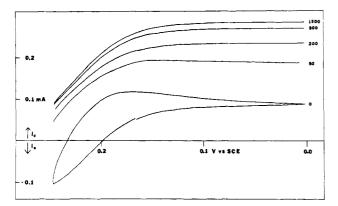
Figure 6. RDE voltammograms at 10 mV/s of a Pt/NAF,TTF<sup>+</sup> electrode in a 10 mM Fe(CN) $_6^{3-}$ , 1 M KBr solution rotated at various speeds. Rotation rates are give in rpm. Electrode area is 0.458 cm<sup>2</sup>.
