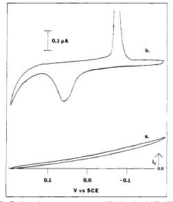
Figure 3. Cyclic voltammograms at 10 mV/s in 10 mM Fe(CN)<sub>6</sub><sup>3-</sup>, 1 M KBr of (a) passivated Ta electrode, (b) Ta/NAF,TTF<sup>+</sup> electrode. Electrode area is 0.049 mm<sup>2</sup>. Note that zero current level is the same for both (a) and (b).
