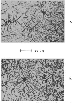
Figure 10. Optical micrographs of  $SnO_2/NAF$ , TTF<sup>+</sup> electrodes that were cycled 10 times in a 1 M KBr solution and removed from solution in (a) the oxidized form, (b) the reduced form.
