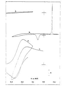
**Figure 2.** Cyclic voltammograms at 10 mV/s in 10 mM Fe(CN)<sub>6</sub><sup>3-</sup>, 1 M KBr of (a) Pt/NAF electrode,  $S = 5 \mu A$ , (b) Pt/NAF,TTF<sup>+</sup> electrode,  $S = 50 \mu A$ , (c) As (b), at higher sensitivity,  $S = 5 \mu A$ , (d) bare Pt electrode, S = 5 A. Electrode area is 0.027 cm<sup>2</sup>.
