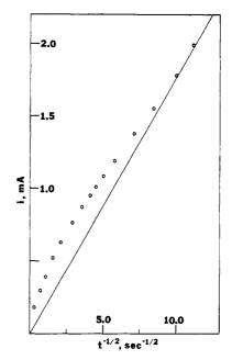
Figure 4. Plot of current vs.  $t^{-1/2}$  for the reduction of ferricyanide on a  $Pt/NAF,TTF^+$  electrode in a 10 mM Fe(CN)<sub>6</sub><sup>3-</sup>, 1 M KBr solution. The potential was stepped from 0.35 to 0.0 V. Electrode area is 0.458 cm<sup>2</sup>.
