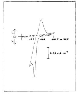
Figure 14. Cyclic voltammogram at 20 mV/s of an n-Si/NAF,TTF<sup>+</sup> electrode in a 1 M KCl solution. Electrode illuminated with a 450-W Xenon lamp at  $\lambda > 590$  nm (—); electrode in the dark (--).
