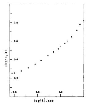
Figure 5. Plot of the ratio of currents observed at a Pt/NAF,TTF<sup>+</sup> electrode (i) and bare Pt electrode ( $i_d$ ) vs. log t. Same experimental conditions as in Figure 4.
