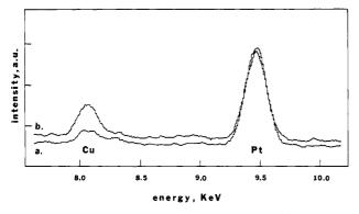
Figure 12. Energy dispersive spectra of a  $Pt/NAF,TTF^+$  electrode that was subjected to copper deposition from an 8.6 mM CuBr<sub>2</sub>, 1 M KBr solution. (a) Spectrum of electrode surface where no TTFBr crystals were present; (b) spectrum of a crystal on the electrode surface.
