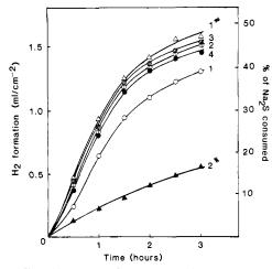
Figure 3. Time dependence of hydrogen production in a 1-cm<sup>2</sup> Nafion film containing CdS and Pt (0.02 mg/cm<sup>2</sup>). The integers are successive runs with the same film. Curves 1# and 2# are for a different film pretreatment. See text for details.
