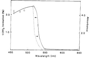
Figure 6. Photoaction spectrum of the CdS-Pt  $(0.04 \text{ mg/cm}^2)$  film (obtained by laser excitation (50 mW)). The dashed line is the UV spectrum of the CdS-Pt film.
