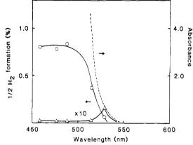
Figure 7. Photoaction spectra of the CdS-Pt (100 Å thick) film (obtained by laser excitation (50 mW)) with irradiation from the Pt side (O) and the bare CdS side ( $\Delta$ ). The dashed line is the UV absorption of the CdS-Pt film.
