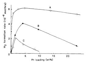
Figure 5. Effect of Pt loading on hydrogen production for different Pt-CdS systems (for 3 h of irradiation). Curve A: chemically reduced Pt:Nafion/β-CdS film. Curve B: photoreduced colloidal Pt-Colloidal CdS. Curve C: sputtered Pt:Nafion/β-CdS film.
