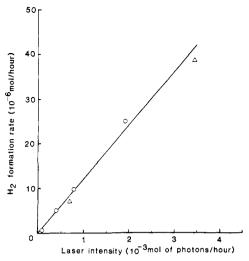
Figure 8. Light-intensity dependence of the rate of hydrogen production in a Nafion film containing CdS and Pt  $(0.04 \text{ mg/cm}^2)$  at 514.5 (O) and 457.9 nm ( $\Delta$ ).
