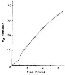
Figure 4. Hydrogen production of the CdS-Pt (0.04 mg/cm<sup>2</sup>)-Nafion film by a low-power (0.15 W/cm<sup>2</sup>) xenon lamp. The dashed line corresponds to a 6-min irradiation by a high-power (1 W/cm<sup>2</sup>) xenon lamp.
