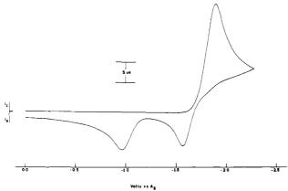
Figure 1. Cyclic voltammogram of 3.71 mM  $[Rh(\mu-t-Bu_2P)(CO)_2]_2$  in THF/0.5 M (TBA)BF<sub>4</sub> scanned between 0.00 and -2.25 V. Scan rate 200 mV s<sup>-1</sup>.
