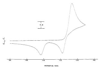
Figure 4. Simulated cyclic voltammograms for an ECE/EEC-Disp mechanism based on  $E^{\circ}_{3} = -1.24 \text{ V}$ ,  $k^{\circ}_{3} = 1.6 \times 10^{-3} \text{ cm s}^{-1}$ ,  $\alpha_{3} = 0.65$ , and the parameters listed for Figure 3. Scan rate and initial and switching potentials are the same as those listed for Figure 1.
