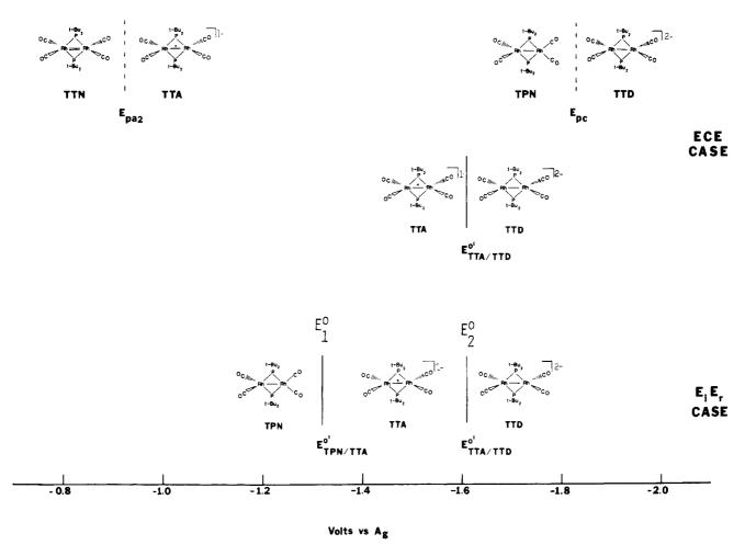
Figure 6. Summary of peak potentials and E° values for the ECE/EEC-Disp and E<sub>i</sub>E<sub>r</sub>-Disp mechanisms. Peak potentials are those observed at 200
