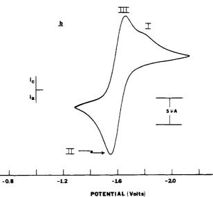
Figure 2. Cyclic voltammograms of 3.71 mM  $[Rh(\mu-t-Bu_2P)(CO)_2]_2$  in THF/0.5 M (TBA)BF<sub>4</sub> scanned between -1.29 and -2.15 V. Scan rate 200 mV s<sup>-1</sup>. (a) First five scans; (b) steady state observed after ca. 10 scans.
