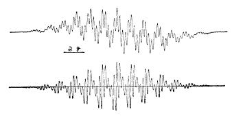
Figure 1. Top: derivative esr spectrum of DPA anion radical produced by electroreduction of  $10^{-3}$  M DPA solution containing 0.1 M tetra-n-butylammonium iodide in N,N-dimethylformamide. Spectrometer conditions: modulation amplitude, 0.1 gauss; power, 10 db; sweep time, 25 min. Bottom: calculated spectrum using constants in text.
