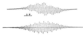
Figure 2. Top: derivative esr spectrum of DPA cation radical produced by treating a  $5 \times 10^{-3} M$  DPA solution in hexane with concentrated sulfuric acid. Spectrometer conditions: modulation amplitude, 0.07 gauss; power, 20 db; sweep time, 25 min. Bottom: calculated spectrum using constants in text.
