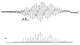
Figure 3. Top: derivative esr spectrum resulting from dilution of solution of DPA cation radical with concentrated sulfuric acid. Spectrometer conditions: modulation amplitude, 0.04 gauss; power, 20 db; sweep time, 25 min. Bottom: calculated spectrum.
