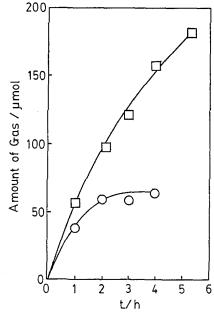
Fig. 1.  $H_2$  evolution from aqueous CH<sub>3</sub>OH and O<sub>2</sub> evolution from aqueous AgNO<sub>3</sub> solutions. Open circles:  $H_2$  from aq. CH<sub>3</sub>OH over Pt (1 wt%)/PbMoO<sub>4</sub>. Open squares: O<sub>2</sub> from aq. AgNO<sub>3</sub> over PbMoO<sub>3</sub>. In both cases, 0.3 g of catalyst was used and the light source was a 200 W high pressure Hg lamp.
