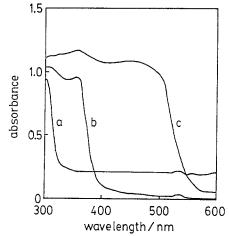
Fig. 2. Diffuse reflectance spectra of (a) PbWO<sub>4</sub>, (b) PbMoO<sub>4</sub>, and (c) PbCrO<sub>4</sub> powders.
