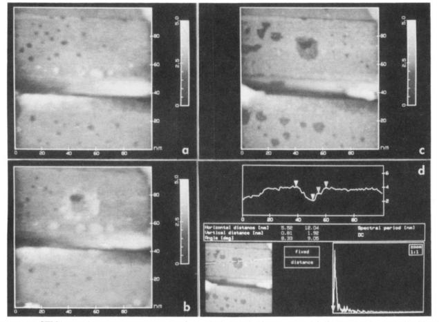
**Figure 1.** (a) STM image of a 100 nm × 100 nm *n*-octadecanethiol film coated on Au/mica. (b) Same area after 15 s of etching ( $V_b = 10 \text{ mV}$ ,  $I_t = 10 \text{ nA}$ ) over a 10 nm × 10 nm area. (c) Same area after 14 min of continuous scanning ( $V_b = 1 \text{ V}$ ,  $I_t = 1 \text{ nA}$ ). (d) Cross sectional view of the pit formed by etching the *n*-octadecanethiol layers.
