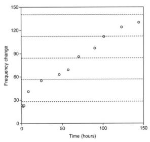
Figure 3. Frequency changes of the crystal during the adsorption of n-octadecanethiols on gold. Dashed lines correspond to the calculated frequency changes for each monolayer formation (up to 4 monolayers) of n-octadecanethiol on gold.
