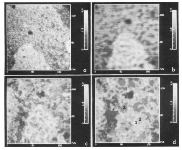
Figure 2. Four sequential STM images (a-d) of a 100 nm × 100 nm area. Time interval between each image is 20 s.  $V_b = 1 \text{ V}$ ;  $I_t = 1 \text{ nA}$ .
