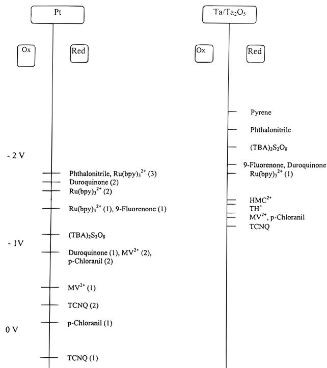
**Figure 4.** Redox potentials in V vs SCE of the compounds studied at the Pt and Ta/Ta<sub>2</sub>O<sub>5</sub> electrodes. Potentials were obtained at a scan rate of 0.1 V/s (see Table 1 for potentials vs Fc<sup>+</sup>/Fc).
