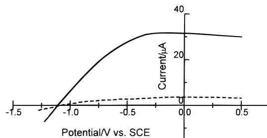
**Figure 2.** Current-potential curves for a Ta/Ta<sub>2</sub>O<sub>5</sub> electrode in 0.1 M TBAP/MeCN (—) under illumination with a 2500 W Xe lamp and (---) without illumination; scan rate = 100 mV/s.
