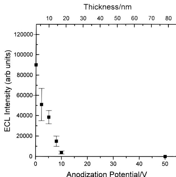
**Figure 9.** ECL intensity for  $\text{TH}^+$  reduction as a function of Ta<sub>2</sub>O<sub>5</sub> thickness. Ta<sub>2</sub>O<sub>5</sub> formed anodically at room temperature in 0.1 M ammonium tartrate. ECL was generated with a 0 to  $-3$  V pulse (10 Hz frequency) in MeCN/0.1 M TBAP, and the signal was integrated for 5 min.
