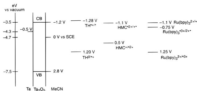
**Figure 10.** Proposed approximate energy levels for Ta/Ta<sub>2</sub>O<sub>5</sub>/MeCN system. All potentials shown are in V vs aq SCE. CB and VB mark the conduction and valence bands from photocurrent measurements. For reference,  $E(\text{Fc}^+/\text{Fc})$  in MeCN = 0.307 V vs aq SCE.
