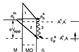
**Figure 11.** Schematic diagram for electron transfer from Ta to solution: (path 1) through Ta<sub>2</sub>O<sub>5</sub> conduction band; (path 2) relaxation in bulk semiconductor (e.g., via traps); (path 3) relaxation via surface states on Ta<sub>2</sub>O<sub>5</sub> or in solution.
