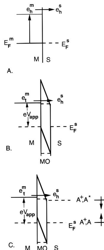
**Figure 1.** Schematic diagram of (A) photoinjection of hot electrons into solution from metal and dark injection (B) through metal/metal oxide interface and (C) with production of an excited state in solution. The Fermi level in solution,  $E_F^s$  is governed by the redox couple  $A^+/A$ .
