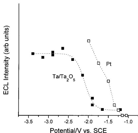
**Figure 8.** ECL intensity of  $\text{Ru}(\text{bpy})_3^{3+}$  (0.5 mM) as a function of the cathodic pulse potential of Pt and Ta/Ta<sub>2</sub>O<sub>5</sub> electrodes. Potential was pulsed between 0 V and the potentials indicated at a cycling frequency of 10 Hz.
