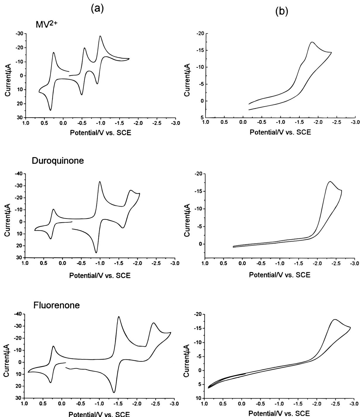
**Figure 3.** Cyclic voltammograms for the reduction of 2 mM  $MV^{2+}$ , duroquinone, and fluorenone in MeCN/0.1 M TBA(PF)<sub>6</sub> at (a) Pt and (b) Ta/Ta<sub>2</sub>O<sub>5</sub> electrodes; scan rate = 0.1 V/s.
