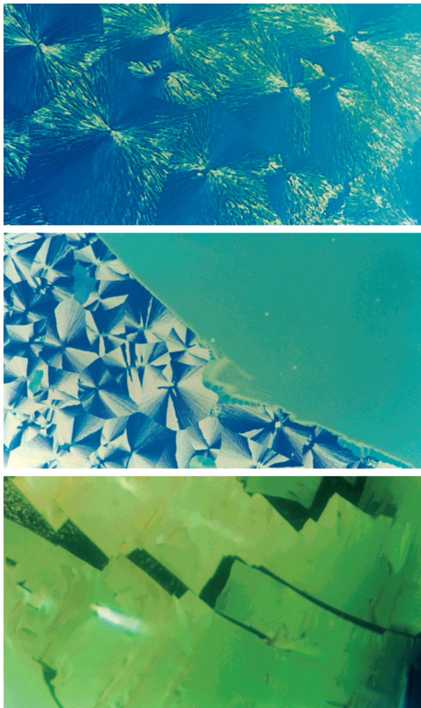
Figure 2. Micrographs of solvent blue 35 crystals between two pieces of glass (area of view, 0.28 \text{ mm} \times 0.49 \text{ mm} ). Top (a): Crystals grown by capillary filling irradiated with polarized light. Middle (b): Crystals first grown by capillary filling and then regrown with the zone-melting technique for upper-right portion (growth rate, 15 \mu\text{m}/\text{min} ) irradiated with polarized light. Bottom (c): Crystals regrown with the zone-melting technique (growth rate, 15 \mu\text{m}/\text{min} ) imaged between two crossed polarizers at a zone at the end of a pass.
