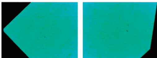
Figure 2. Images ( 0.15 \text{ mm} \times 0.12 \text{ mm} ) of \text{Ru}(\text{bpy})_3(\text{ClO}_4)_2 single-crystal thin films (about 1.5 \mu\text{m} thick) between two crossed polarizers with an optical microscope. Dark areas are open air spaces. The two corners on the single crystal are 90^\circ and 140^\circ .
