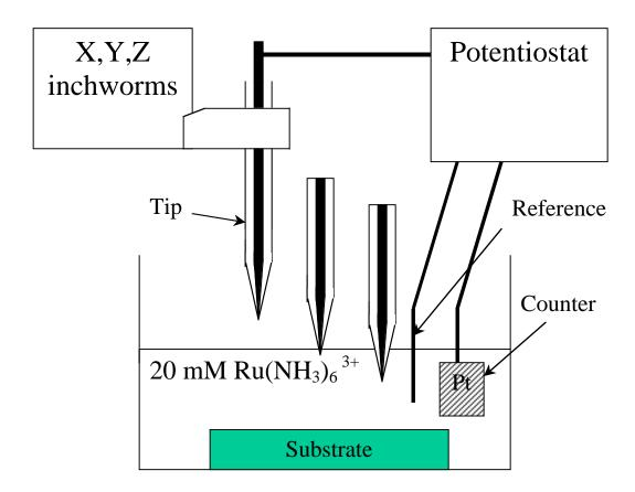
**SI Figure 1.** Schematic diagram of the experimental setup for the electrochemical approach at air/solution interfaces.
