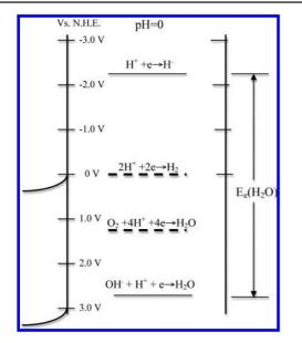
*Figure 9.* More realistic schematic of the bands in  $TiO_2$  and water (solid lines). The dashed lines are the thermodynamics for the multielectron reactions that require electrocatalysts.
