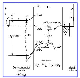
*Figure 8.* Typical semiconductor band diagram with respect to thermodynamic (multielectron transfer) half-reactions in solution for water splitting for SrTiO<sub>3</sub>/solution/Pt photoeletrochemical cell. Adapted with permission from Nozik, A. J.; Memming, R. *J. Phys. Chem.* **1996**, *100*, 13061. Copyright 1996 American Chemical Society.
