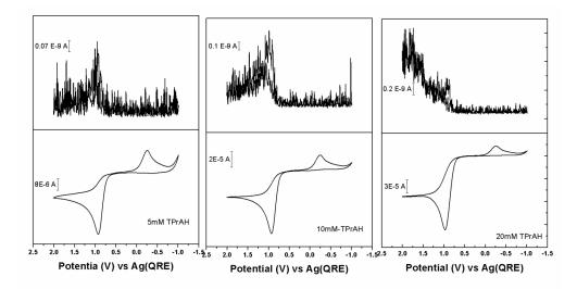
**Figure S1.** CV and ECL curves of various concentrations of TPrAH in a 0.1 M TBAPF<sub>6</sub> MeCN solution on Pt electrode with aerated conditions.
