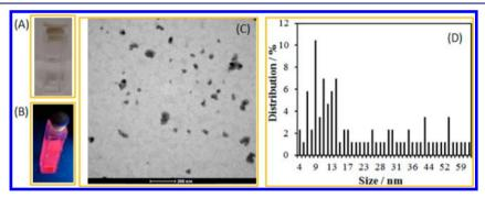
Figure 4. Photographs of 1a organic nanoparticles in water under (A) ambient and (B) UV light. TEM results (C) and size distribution (D) of 1a organic NPs. The density of 1a NPs used in the TEM is  $\sim 10^{-5}$  g/cm<sup>3</sup>.
