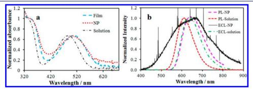
Figure 5. (a) Normalized absorbance of 7  $\mu$ M 1a solution in DCM, 1a film, and 1a NPs in water. (b) Normalized PL spectrum of 1a NPs in water, and ECL spectrum of 1a NPs in water generated with 100 mM  $K_2S_2O_8$  as coreactant. Normalized PL and ECL spectra of 1a solution in DCM are shown for comparison.
