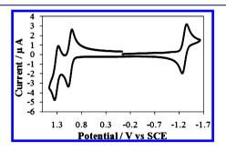
Figure 1. CV of 0.5 mM 1a in DCM with 0.1 M TBAPF<sub>6</sub>. Scan rate = 100 mV/s; area of electrode =  $0.028 \text{ cm}^2$ .
