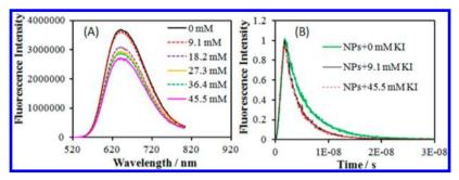
Figure 6. (A) Fluorescence spectra of 1a organic NPs without KI and in the presence of KI at different concentrations. (B) Fluorescence decay profiles of 1a organic NPs before and after addition of KI. The decay profiles for KI concentrations ranging from 9.1 to 45.5 mM are overlapped. Error in fluorescence intensity = 1%; error in fluorescence lifetime = 0.9%.
