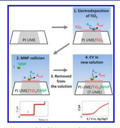
**Figure 1.** Schematics of the fabrication and the characterization of T-UME by electrodeposition of  $TiO_2$  on Pt UME, collision with MNP, removal of UME from the solution, and running CV in new solution without additional MNPs.
