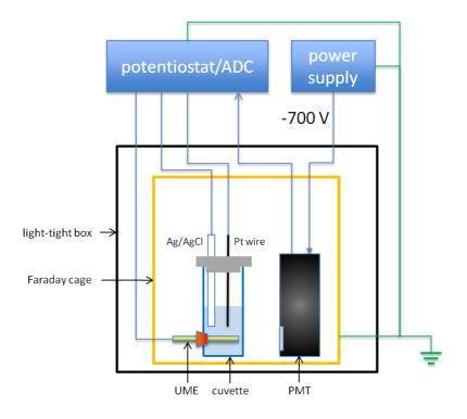
Figure S1. Schematic of the experimental setup used to measure the current and ECL signal of single droplet collision.
