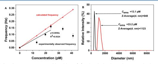
Figure 8. (A) Collision frequency vs. concentration of the cyclohexane (Fc) emulsion droplet. The error bars correspond to the standard deviation at three measurements. The potential was held at +0.6 V vs. the Ag wire. (B) DLS data with different concentrations of the cyclohexane (Fc) emulsion droplet.
