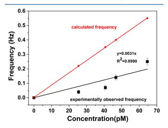
Figure 5. Collision frequency as a function of concentration of the benzene (ZnTPP) emulsion droplet. The error bars correspond to the standard deviation at three measurements. The potential was held at +0.65 V vs. Ag wire.
