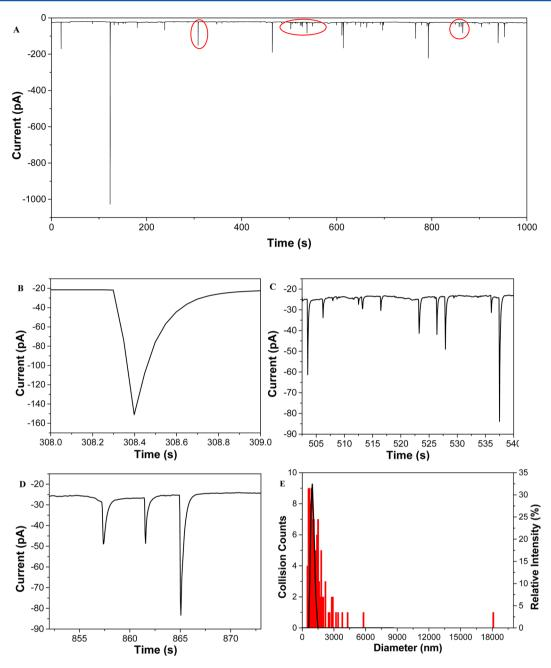
**Figure 6.** (A) Amperometric i-t curve of the emulsion droplet collisions on the Au UME. The test sample contains ca. 19.8 pM cyclohexane (Fc) emulsion droplets and cyclohexane saturated water. (B–D) Magnified i-t curves showing clear spiked responses. The Au UME was biased at +0.6 V vs. Ag wire during the entire experimental time. (E) Comparison of the droplet size distribution from eq 3 (red bars) with DLS data (black line).
