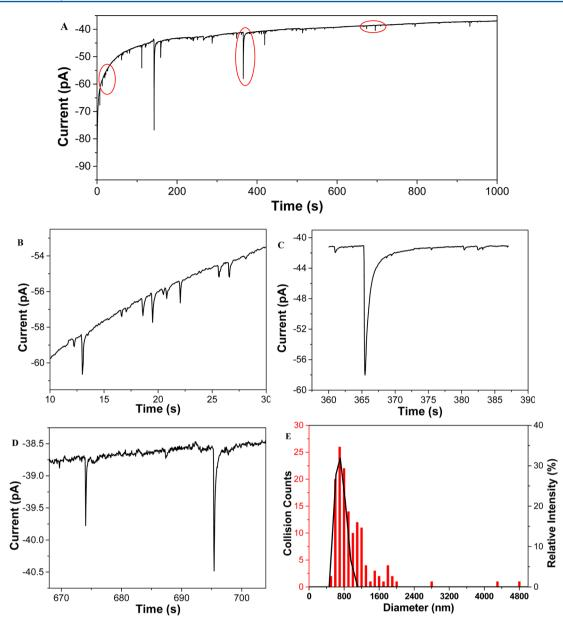
**Figure 3.** (A) Amperometric i-t curve of the emulsion droplet collisions on the Au UME. The measurement mixture contains ca. 46.7 pM benzene (ZnTPP) emulsion droplets in benzene-saturated water. (B–D) Magnified i-t curves showing the clear spike-type responses. The Au UME was biased at +0.65 V vs. Ag wire during the entire experimental time. (E) Comparison of the droplet size distribution from eq 3 (red bars) vs. the DLS data (black line).
