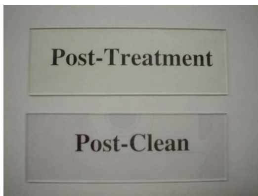
Figure 9.4: Photograph of the ITO slides before and after mechanically cleaning. The “post-treatment” sample is hazy with loosely bound material. After cleaning, the “post-clean” sample is transparent.
